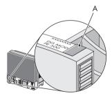
5. Dock the DC lid at an angle, and attach. The captive screws must protrude.
