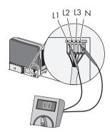
8. Verify the absence of voltage in L1, L2 and L3 against PE at the AC terminal.If voltage is present, check the installation.
