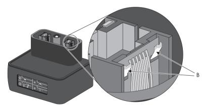
You must replace the handle of the Electronic Solar Switch before restarting the inverter. You can obtain replacement handles for the Electronic Solar Switch from your specialist dealer (see Section 15 "Accessories", page 125).
