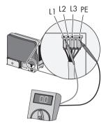
9. Verify the absence of voltage in the multi-function relay against PE at all terminals.
