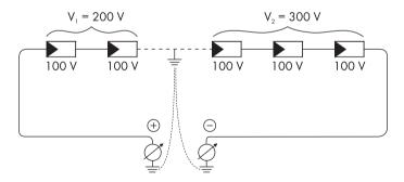
In this case, the earth fault is between the 2nd and 3rd PV modules.
