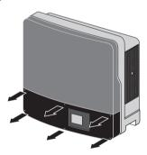
6. To remove the lower enclosure lid, lift it up from the bottom
