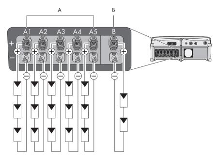
Up to 4 strings (Sunny Tripower 8000TL/10000TL/12000TL) or 5 strings (Sunny Tripower 15000TL/17000TL) can be connected at input area A. One string can be connected at input area B.
