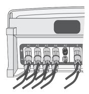
7. Ensure that all DC connectors are securely in place.
