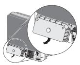
4. Remove all surge arresters from the slots. To do this, compress the grooved areas on either side.
