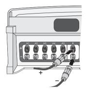
5. After connecting the string, watch out for messages in the display and any acoustic signals.
