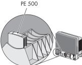
If surge arresters are only required for input A, the two surge arresters must be mounted on the two upper slots.
