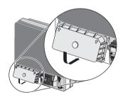
9. Pre-screw all 4 screws of the DC lid and then tighten them (torque: 3.5 Nm).
